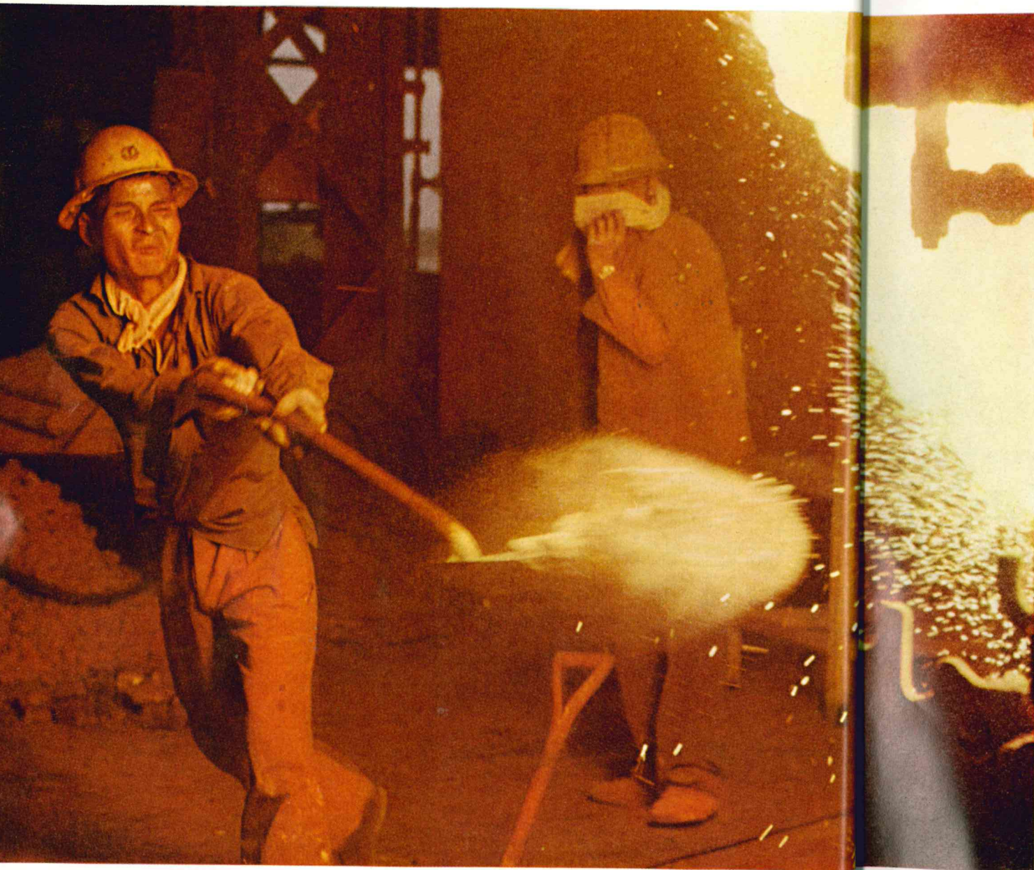
Searing belch of a blast furnace erupts as a workman tosses in another shovelful of lime. The Taiwan Iron Manufacturing Corporation in Taipei produces pig iron, foundry products, and steel from scrap purchased abroad. Unlike some other developing lands, Taiwan has deferred constructing a large-scale modern steel mill, preferring to concentrate its effort and money on agricultural reform. Says the author: "Taiwanese reason, 'We have to learn to feed our people first, then we'll have a steel mill.' " The government has now approved plans for a giant steel plant to be built within the next few years.
